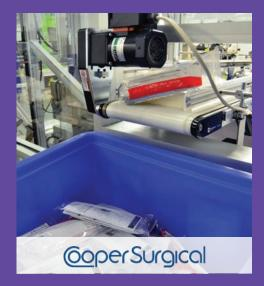
Sometimes it takes a mix of standard conveyors and custom engineered solutions to move product exactly where it needs to be. We helped CooperSurgical maximize floor space by using a series of overhead conveyors to move cervical sampling spatulas across their facility.
