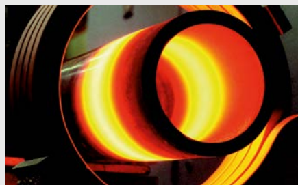
Inductively heated pipe
