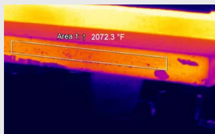
Run-off area of a continuous casting plant
