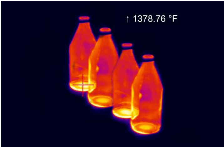
Hot spot detection at glass bottle production
