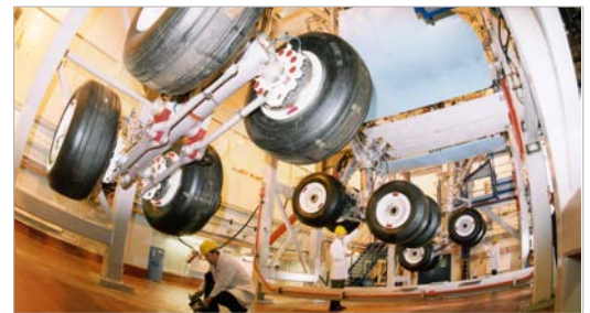
Airbus UK landing gear test rig. Clamp-on sensors were installed to measure the flow of the hydraulic oil in the landing gears.
